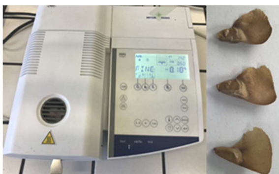
Fig. 4. Determination of moisture content by Moisture Analyzer (Mettler-Toledo AG, Laboratory & Weighing Technologies, Greifensee, Switzerland)
